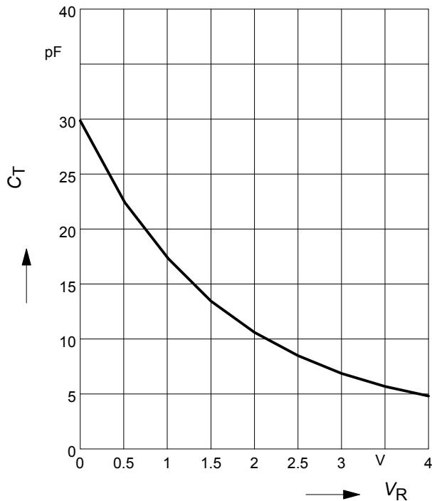
**Normalized diode capacitance**
