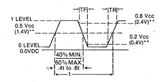
"0" Level =  $0.1 \text{ Vcc } (0.4\text{V})^{**} \text{ max.}$
