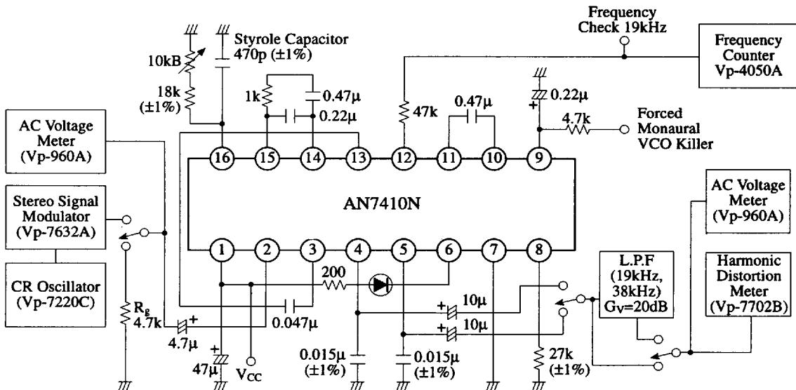
Note 1) VCO free-run frequency is adjusted to 19kHz (±10Hz) with frequency check terminal.
