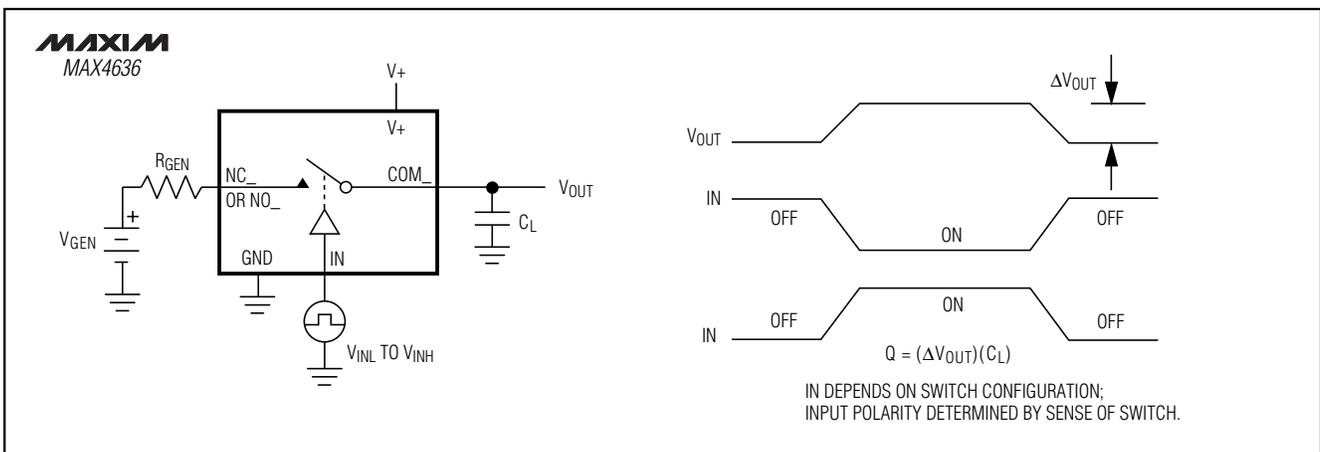
Figure 2. Charge Injection
