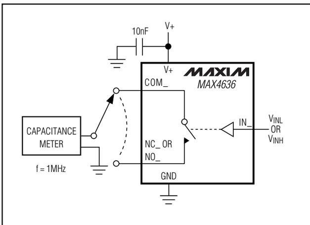
Figure 3. Channel Off/On-Capacitance
