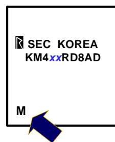
b. Top marking example of mirrored package
