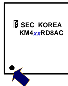
b. Top marking example of normal package
