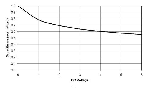
Figure 2. Typical Diode Capacitance VS. Input Voltage (normalized to 0Vdc)
