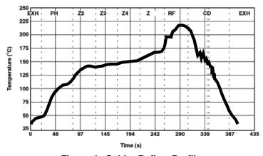
Figure 4. Solder Reflow Profile
