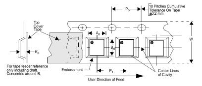
Figure 5. Tape and Reel Mechanical Data
