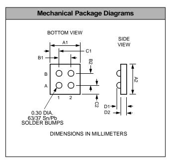
**Package Dimensions for** CSPESD301/302/303 Chip Scale Package
