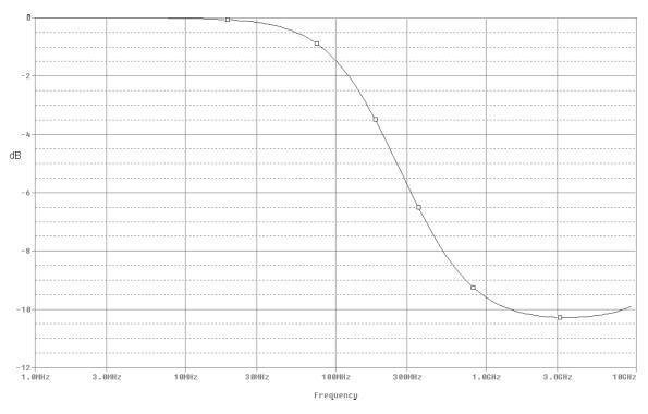
Figure 1. Typical EMI Filter Performance (Simulated)
