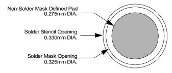
Figure 3. Recommended Non-Solder Mask Defined Pad Illustration
