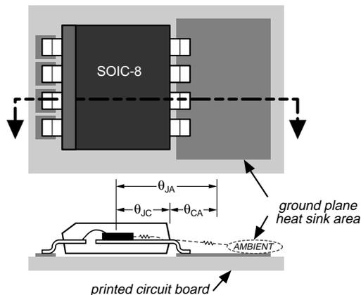
**Figure 3. Thermal Resistance**
