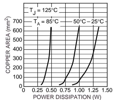
**Figure 5. Copper Area vs. Power-SOIC Power Dissipation**
