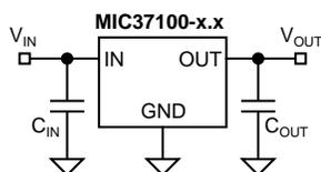
Figure 1. Capacitor Requirements
