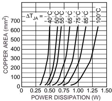
**Figure 4. Copper Area vs. Power SO-8 Power Dissipation**
