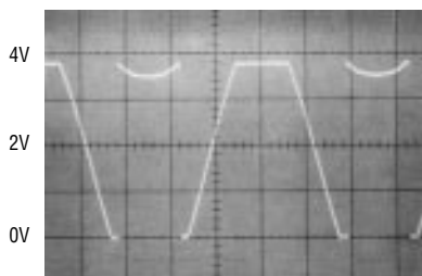
LM324, LM358, OP-221 EXHIBIT OUTPUT PHASE REVERSAL
