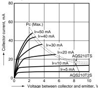
4-2. Collector current vs. voltage between collector and emitter characteristics (Ic-VcE) Measured portion: between terminals 6 and 7 (AQS210TS), (AQS210TS)
