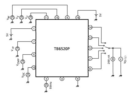
Input amplitude 1.5 to 3.5 V to V<sub>U</sub>, V<sub>V</sub>, V<sub>W</sub>, V<sub>IP</sub>, V<sub>CMP</sub>, and V<sub>OC</sub>, and cause the output to function. TEST CIRCUIT 9:  $V_{AD(L)}$ ,  $V_{AD(H)}$
