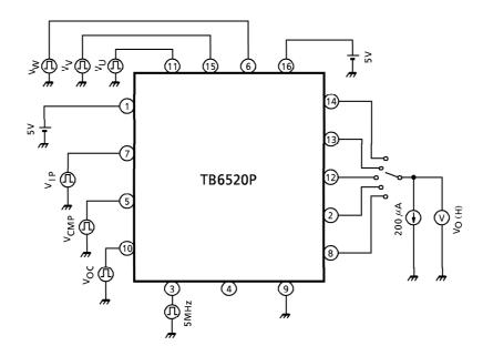
Input amplitude 1.5 to 3.5 V to V<sub>U</sub>, V<sub>V</sub>, V<sub>W</sub>, V<sub>IP</sub>, V<sub>CMP</sub>, and V<sub>OC</sub>, and causes the output to function.
