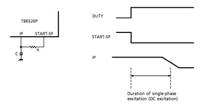
Setup example : C = 4.7  $\mu$ F $_{\times}$  R = 220 k $\Omega$
