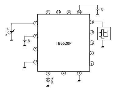
$\bullet$  Change  $V_{\mbox{\scriptsize DUTY}}$  and measure Ton.
