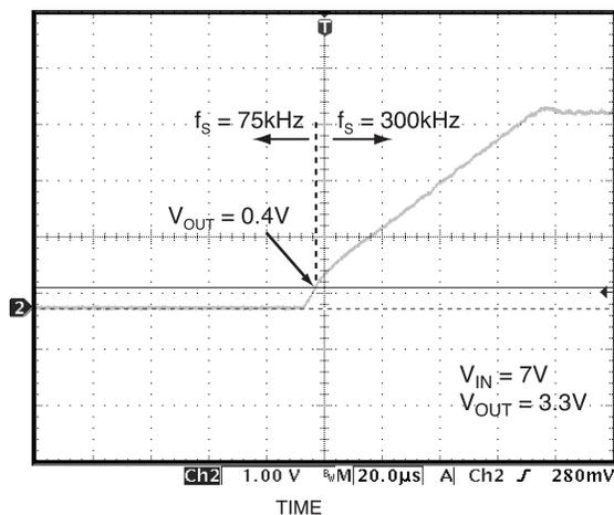
Figure 4. Startup Waveform
