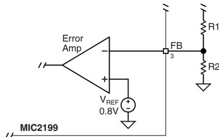
**Figure 6. Voltage-Divider Configuration**
