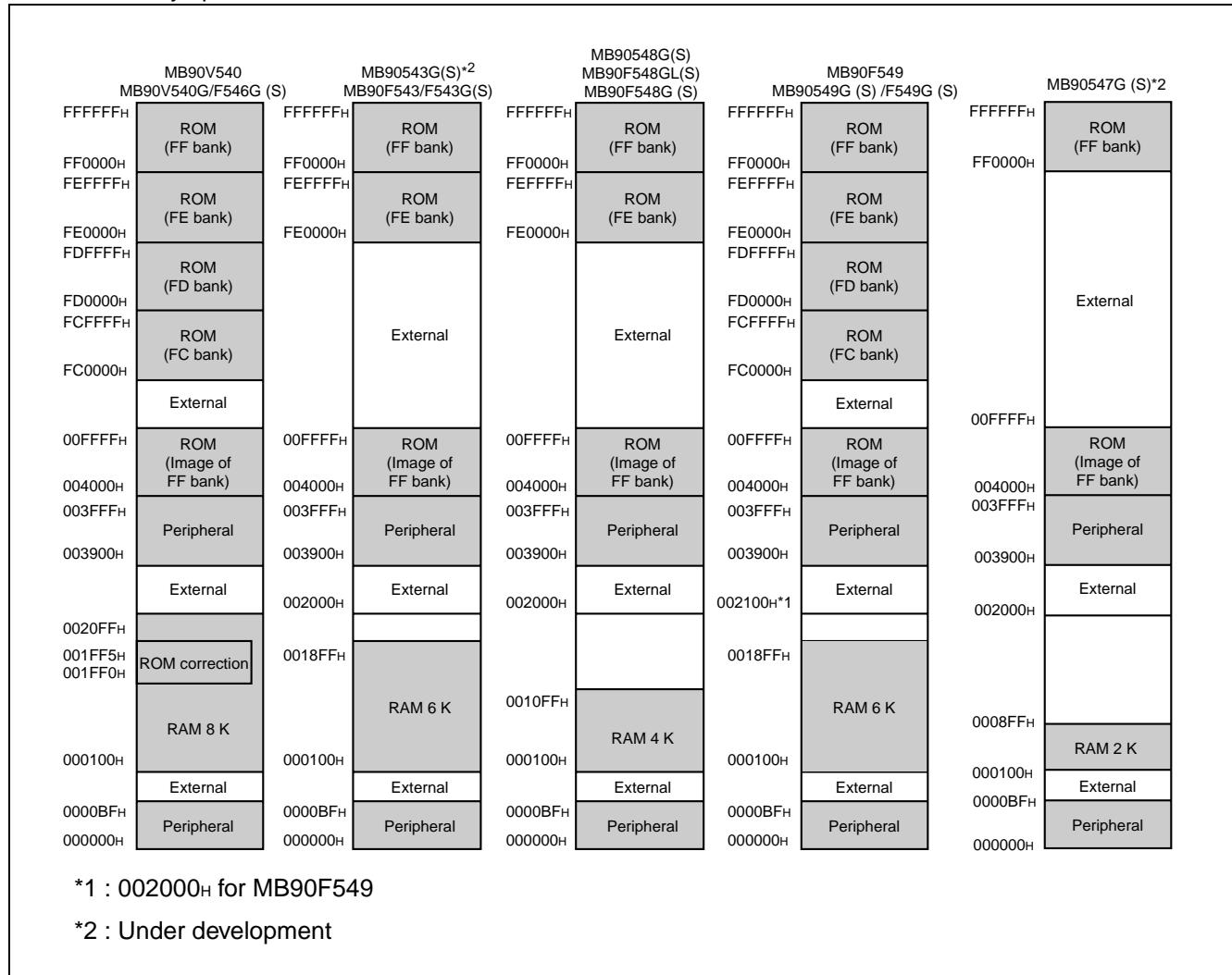
Note : The high-order portion of bank 00 gives the image of the FF bank ROM to make the small model of the C compiler effective. Since the low-order 16 bits address are the same, the table in ROM can be referenced without using the "far" specification in the pointer declaration.
