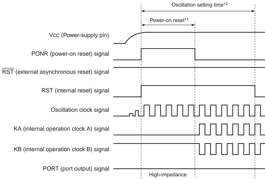
\*1 : Power-on reset time : Period of “clock frequency  $\times 2^{17}$ ” (Clock frequency of 16 MHz : 8.19 ms)
