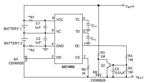
$^*C_{\text{TC}}$  &  $C_{\text{TD}}$  are optional for delay time adjustment.
