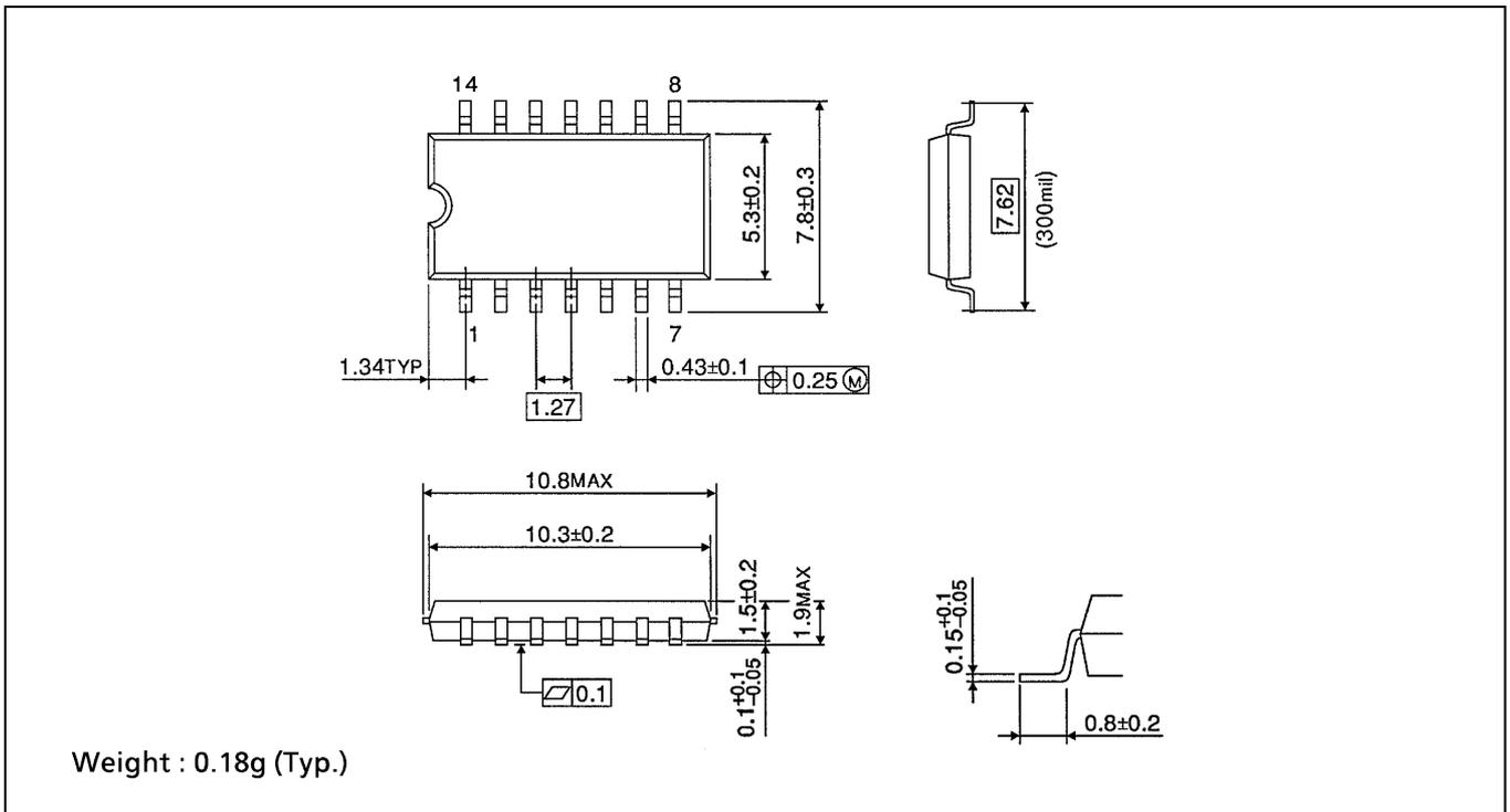
**SOP 14PIN (150mil BODY) PACKAGE DIMENSIONS (SOP14-P-150-1.27)**
