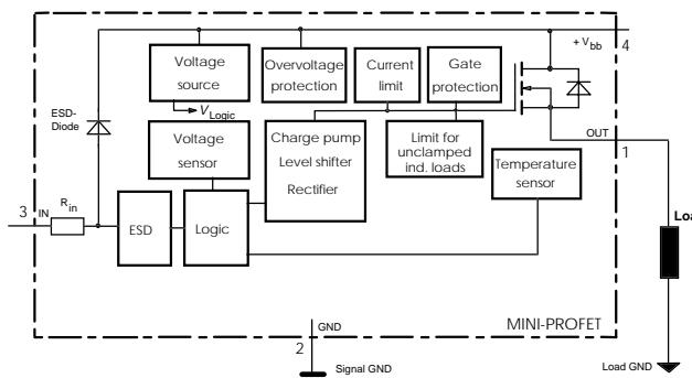
1) With resistor  $R_{GND}=150 \Omega$  in GND connection, resistor in series with IN connections reverse load current limited by connected load.
