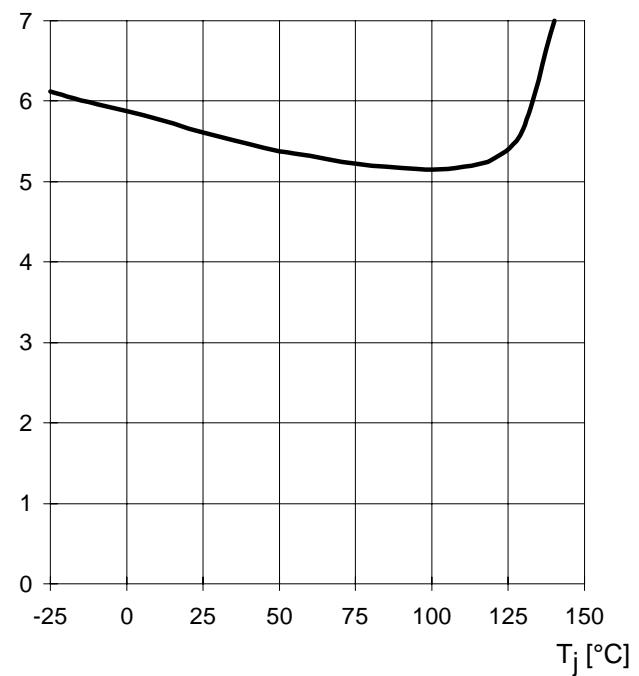
**Typ. input turn on voltage threshold**
