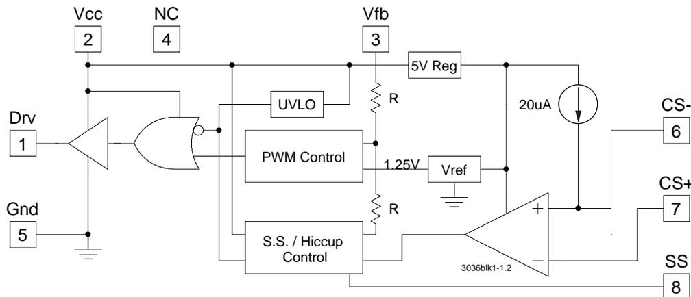
Figure 1 - Simplified block diagram of the US3036
