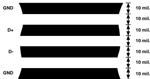
Figure 10. Arrangement of Signal Tracks
