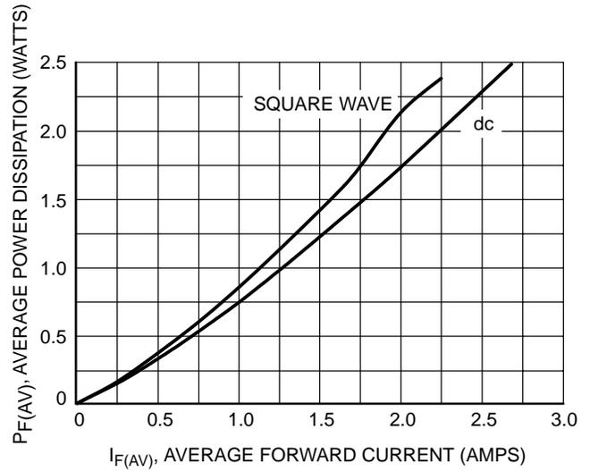
**Figure 6. Power Dissipation**
