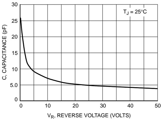
**Figure 7. Typical Capacitance**
