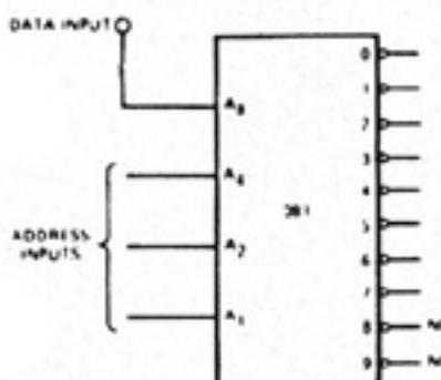
If data is applied to the A<sub>8</sub> input in the octal decoding mode, the outputs 0 through 7 selected by A<sub>1</sub>, A<sub>2</sub> and A<sub>4</sub> will have the same states as the data. Thus, the serial output of an 8-channel multiplexer may be demultiplexed by using A<sub>1</sub>–A<sub>4</sub> as address inputs synchronized with the multiplexer channel-select signals.
