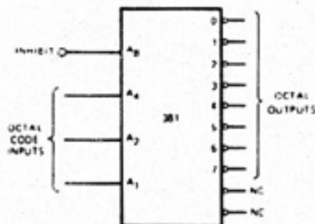
Since outputs 8 and 9 are continuously high if the A<sub>8</sub> input is low, grounding A<sub>8</sub> converts the 381 to an octal decoder.
