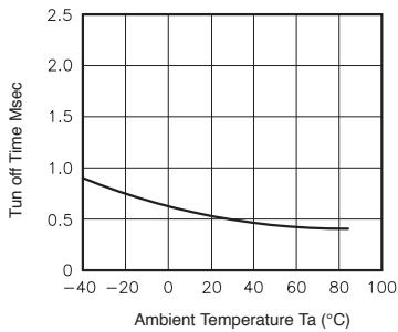
**Fig.5** LED operate vs. ambient temperature
