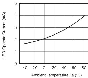
**Fig.6** LED turn off current vs. ambient temperature
