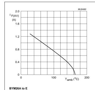
a = 1.42;  $V_R = V_{RRMmax}$ ;  $\delta = 0.5$ . Device mounted as shown in Fig.19. Switched mode application.
