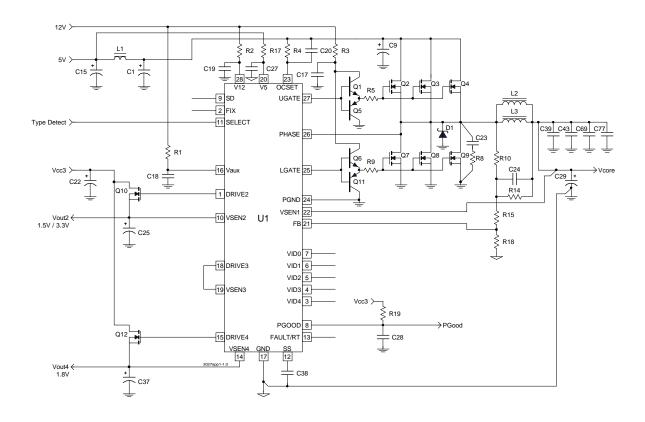
Figure 2 - Typical application of US3027 for the AMD Slot A socket
