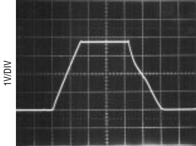
A_V = 1 100\mu s/DIV C_L = 12pF INPUT PULSE = 0V TO 3.8V LT2178/79 • TPC14
