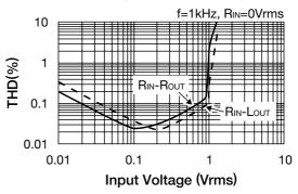
5. THD of output signal – Input voltage (QSrround) 6. Input voltage (1) – Power supply voltage (QSrround) f=1kHz, The signals that are inputted in Lin and Rin are out out of phase and same amplitude.
