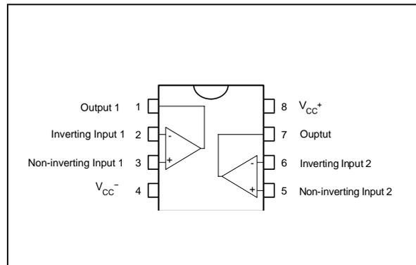
**SCHEMATIC DIAGRAM** (for 1/2MC33172)
