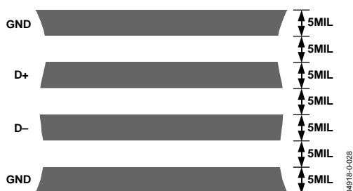
Figure 29. Arrangement of Signal Tracks
