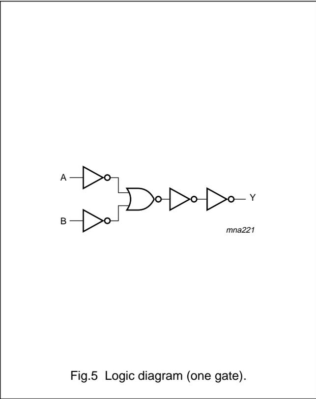
Fig.5 Logic diagram (one gate).
