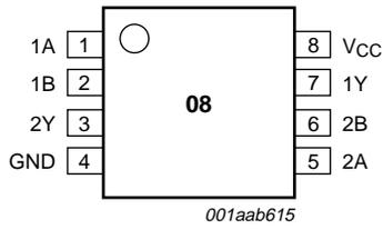
Fig.1 Pin configuration TSSOP8 and VSSOP8.
