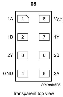
Fig.2 Pin configuration XSON8.
