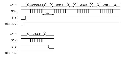
Cautions 1. Wait time twait (1  $\mu$ s) is necessary from the rise of the 8th shift clock of command 1 until the fall of the 1st shift clock of data 1.
