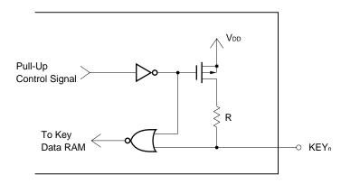
In the event of key source output, the pull-up control signal becomes "H", and the pull-up transistor is turned on.
