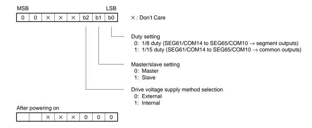
**Note** When multiple chips are used, only the chip that sent the command is enabled. If initialization is performed during display, the display may be affected (especially when multiple chips are used).
