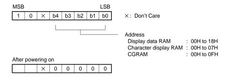
**Note** If an unspecified address is set, data cannot be written until a correct address is next set. The address is not incremented even in increment mode.
