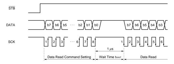
Caution As the DATA pin is an Nch open-drain output, a pull-up resistor must be connected externally. (1 k $\Omega$  to 10 k $\Omega$ )
